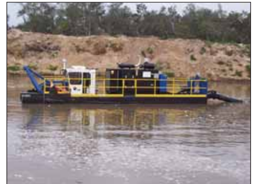
A Model 7012 HP removes sand from a sand mine in Eastern Florida.
